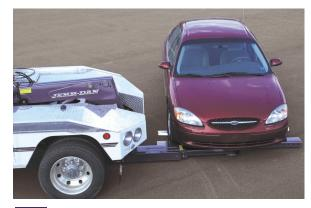
The operator closes the L-arms activating the patented over-center L-arm LOCKLINK. At this moment, both grid boxes expand outward until they gently contact the front tires. When the car is raised this unique action will center the car to the crossbar pivot.
