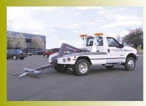
**Power Tilt Lifting Boom** - The power tilt boom can also be tilted down to 10°. Not all QUICK-PICKS<sup>®</sup> occur on flat parking lot surfaces.
