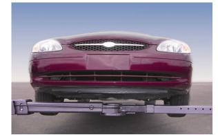
**6** The car is ready to be towed. Notice the clearance around the low-profile height crossbar and how the crossbar is positioned in the middle of the car.
