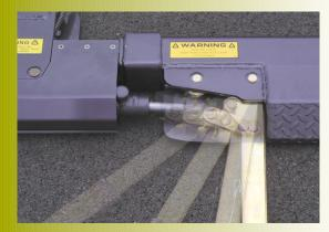
Adjustable L-Arm LOCKLINK - As the adjustable L-Arm closes, the LOCKLINK attaching the L-arm cylinder to the L-Arm rotates into an over-center position. The adjustable L-Arm is now locked in the closed position and cannot be forced open by a loss of hydraulic pressure.
