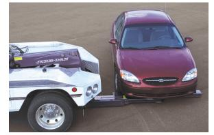
The operator continues backing straight until the crossbar contacts the driver's side tire. It is not necessary for the driver to precisely center the crossbar pivot. QUICK-PICK<sup>®</sup> does that for him.
