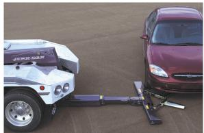
With the stinger extended and L-arms opened and adjusted for tire size the operator properly positions the wrecker
