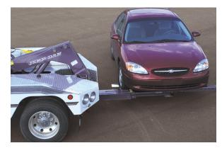
**5** The operator now raises the stinger and up comes the front of the car. Notice how the cross-bar pivot is now centered with the vehicle.
