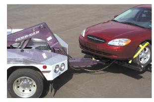
**?** The operator properly retracts the stinger and adds all appropriate towing and safety attachments.
