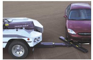
The operator moves the wrecker straight back. The crossbar contacts the passenger side tire and begins to pivot.
